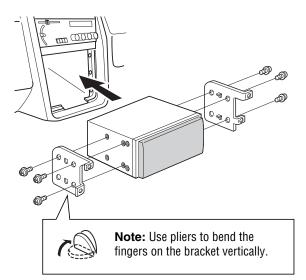
Select mounting screws according to the hole positions and hole shape of the bracket.
